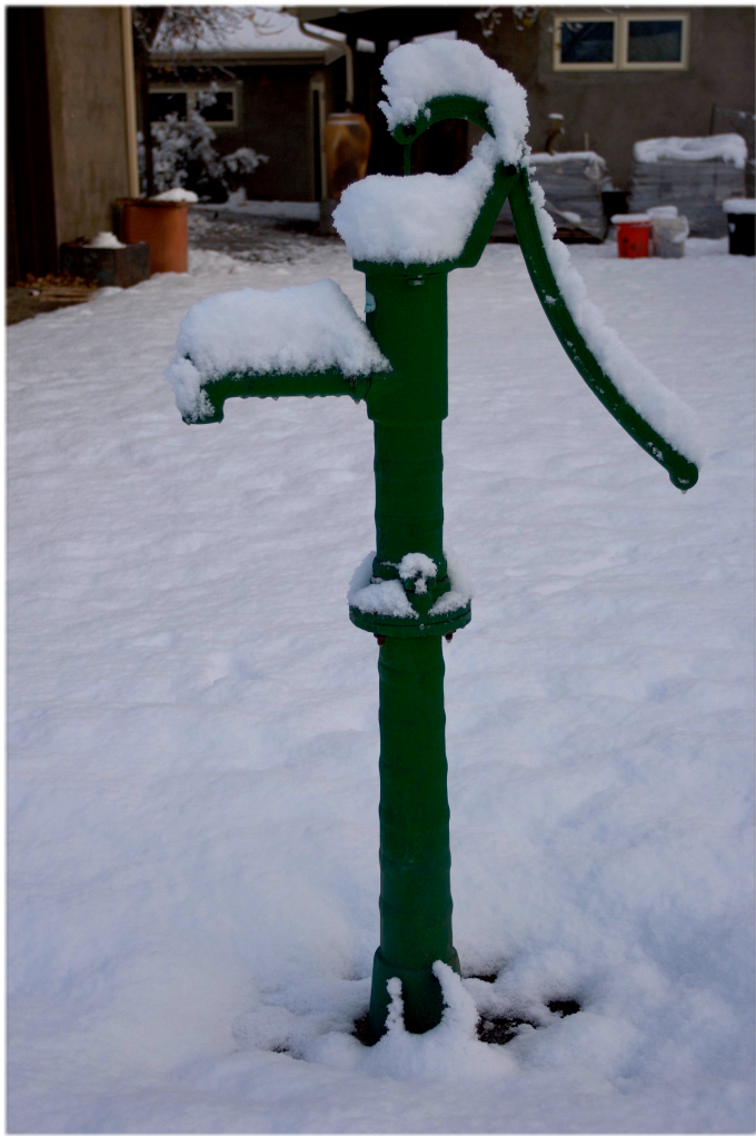
Pumping water from an underground cistern does not have to involve electricity. It can be quite rustic and involve relatively little labor.
