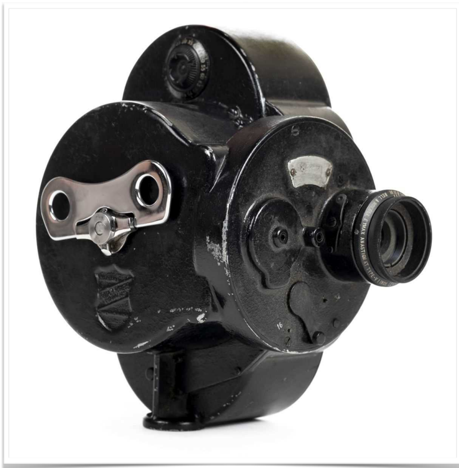
1927 Eyemo 35mm Camera. This is one of the cameras used on this expedition, it had a 100 foot film capacity. When wound up the camera would run for about 20 seconds at 24 frames per second. It could also be "hand cranked". 100 feet of film will last about a minute.
